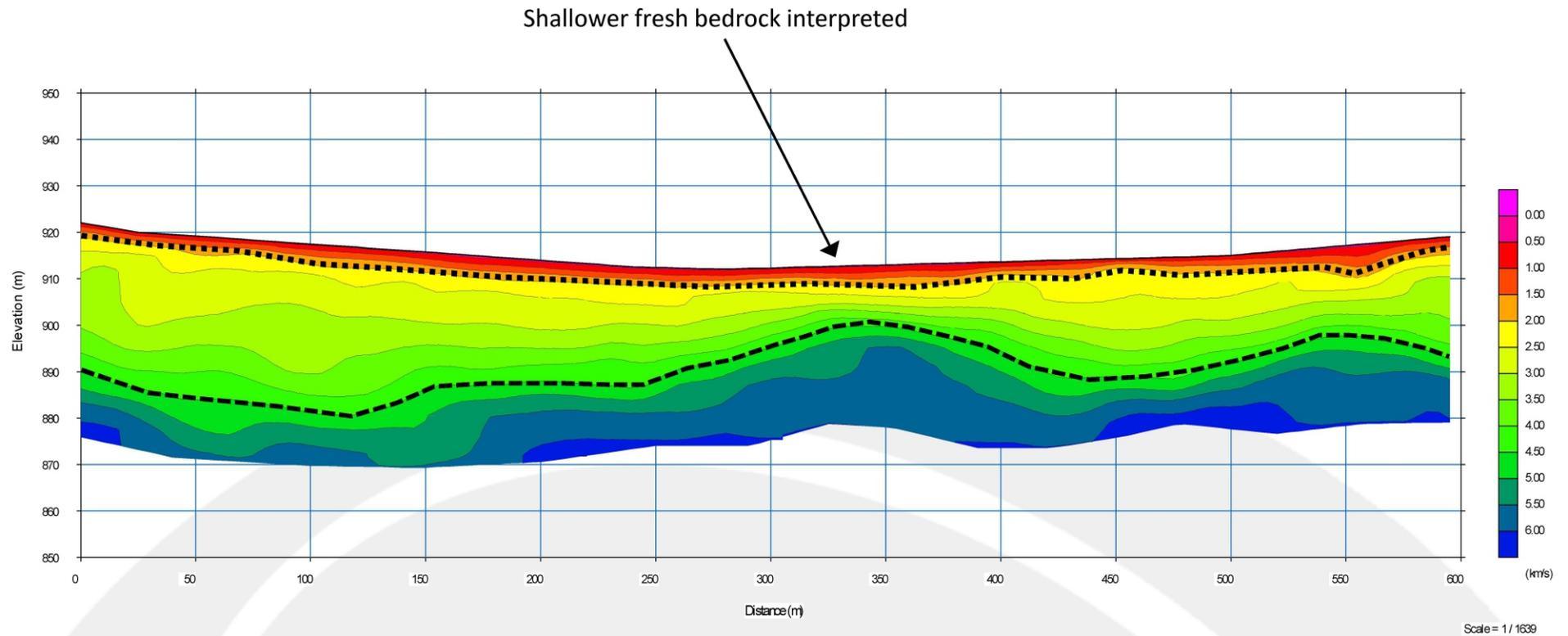
**FIGURE 11: Traverse Q1Q2 Seismic Tomography Model (Smithfield Dam Site)**
