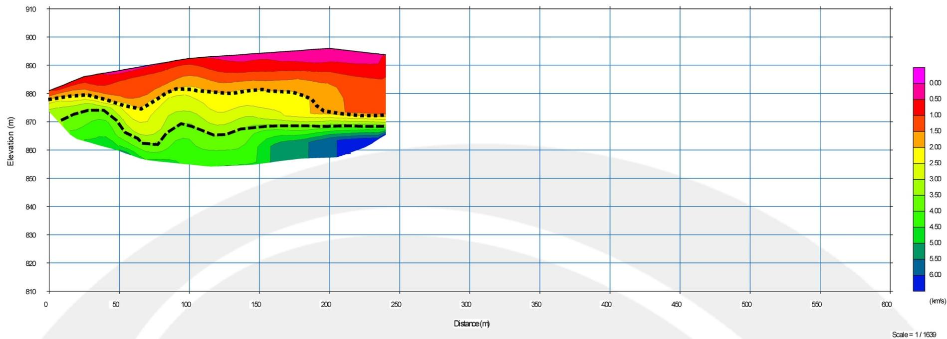
**FIGURE 16: Traverse R1T2 Seismic Tomography Model (Smithfield Dam)**
