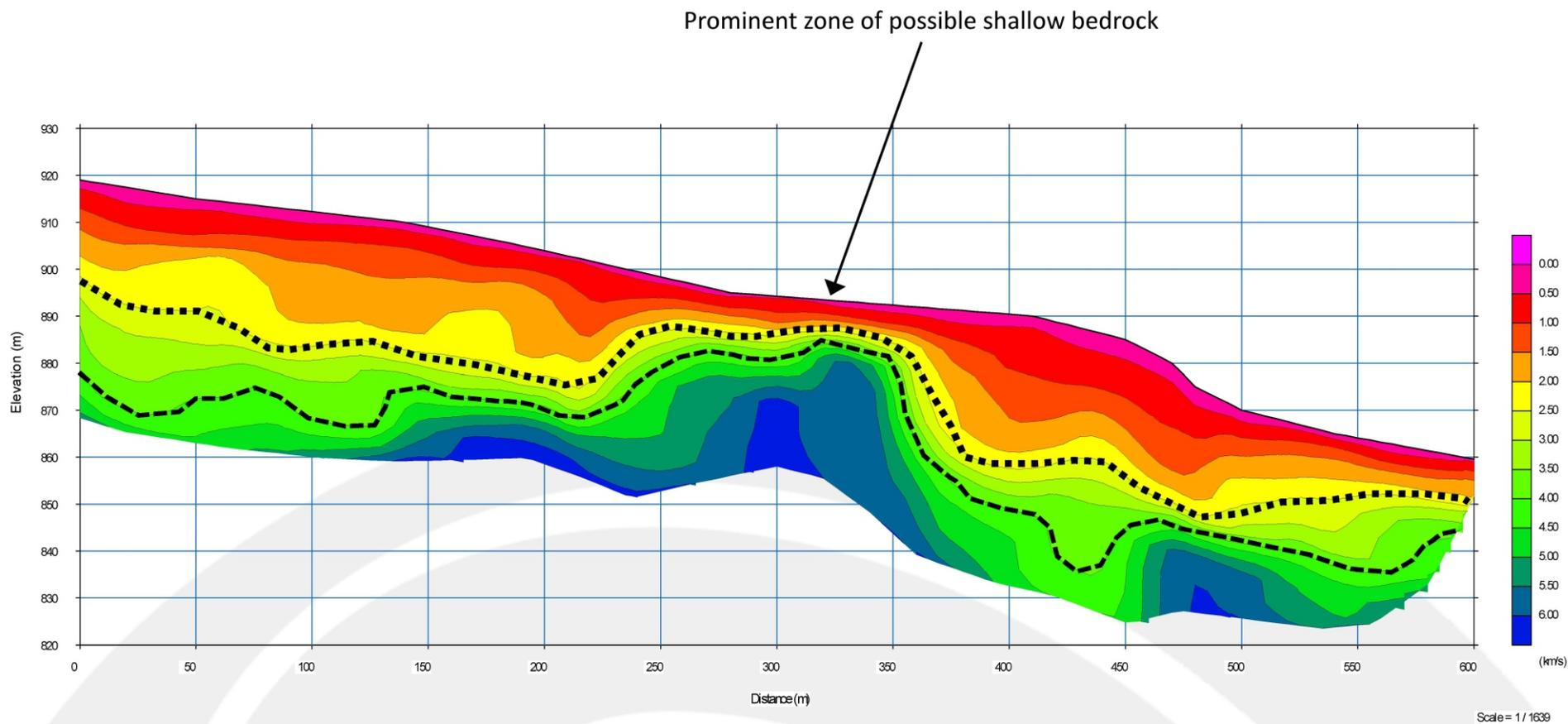
**FIGURE 18: Traverse L1L2 Seismic Tomography Model (Smithfield Dam)**
