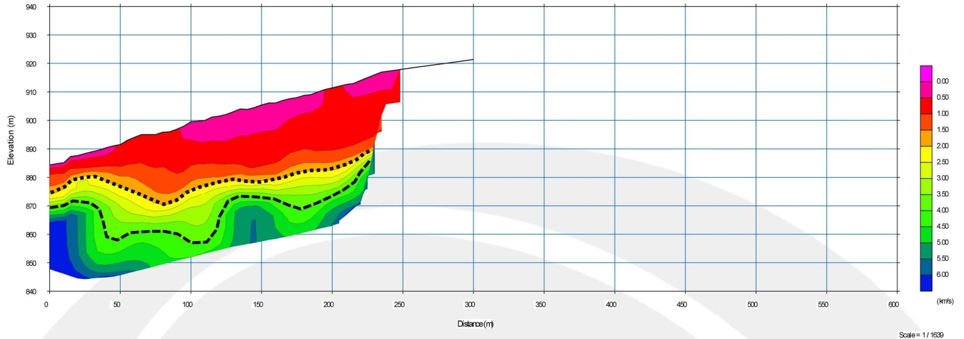
**FIGURE 24: Traverse O1O2 Seismic Tomography Model
